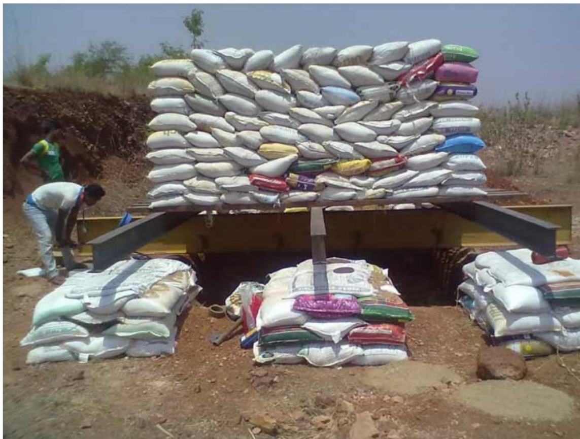
Gravity Loading Method
